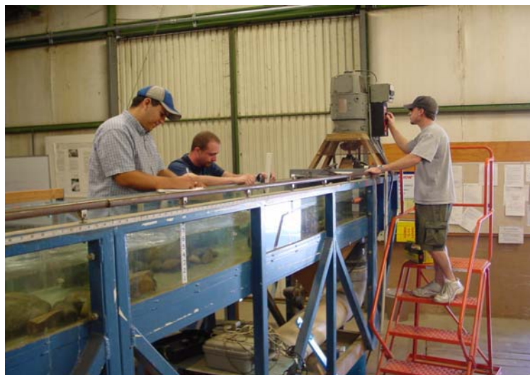
Figure 20. Water velocities being measured within longitudinal displacement flume
