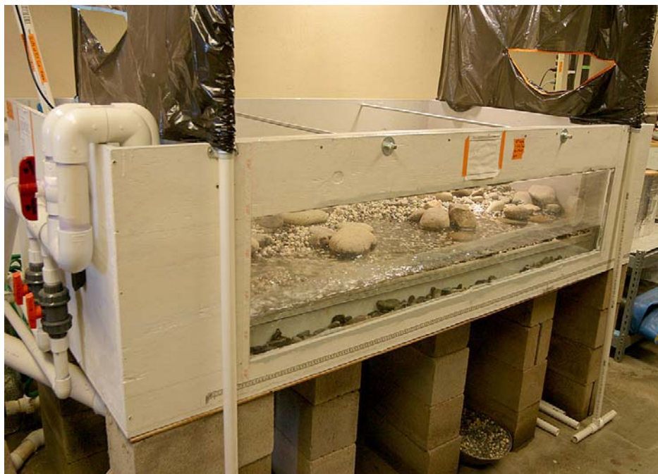
Figure 26. The lateral displacement flume during an experiment. Note the main channel in front of the simulated bank habitat.
