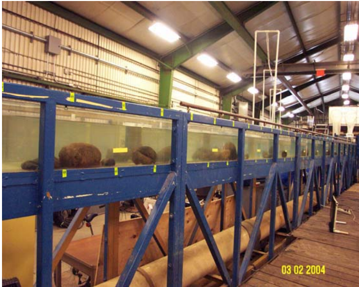
Figure 19. The longitudinal displacement flume outfitted with rocks from the South Fork of the American River
